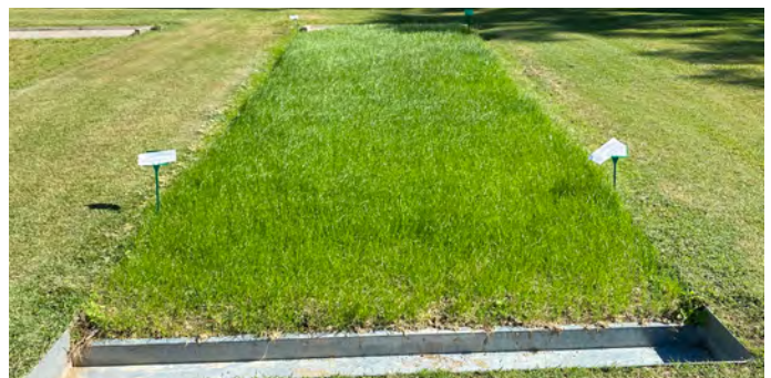
Hydromulch after watering and grass establishment (Source: Healthy Land & Water).
