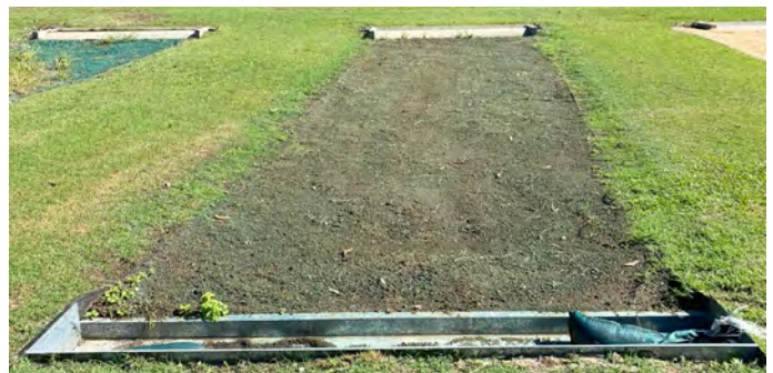
Spray on soil binder (polymer) (Source: Healthy Land & Water).
