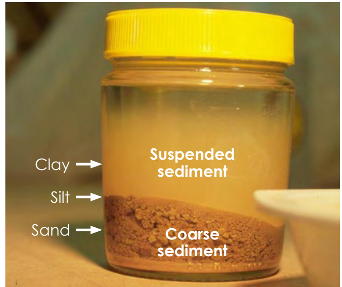
Sediment particle sizes (Source: Catchments & Creeks).
